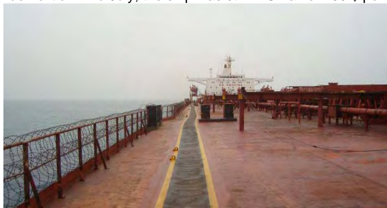
Enhanced anti piracy protection on Front Climber's deck , March 2012 © V Basko
