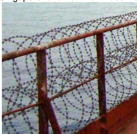
Enhanced anti piracy protection on Front Climber's deck , March 2012 © V Basko
