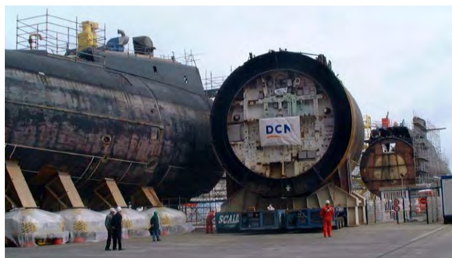
Removal of a reactor unit © DGA
