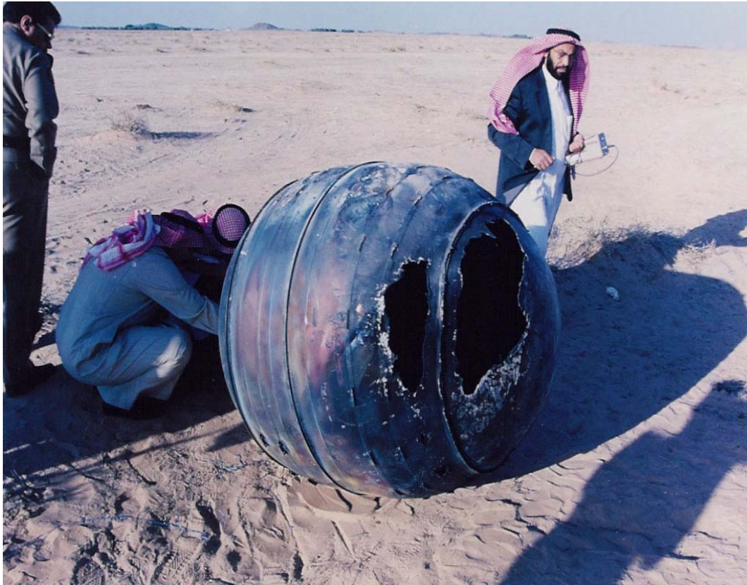
Titanium tank weighing around 50 kg from the 3 rd stage of the Delta 2 launcher, which fell on 21 January 2001 in Saudi Arabia after eight years in orbit. Photo by NASA Orbital Debris Program Office.
