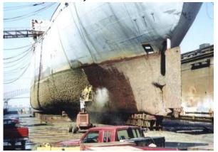
Cleaning of the hull during 1999 dry dock (Corps photo)
