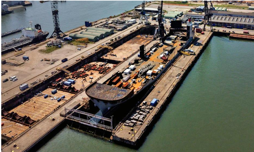
The Fremantle Highway , August 2024, after removal of the upper decks. © Olivier Middendorp
